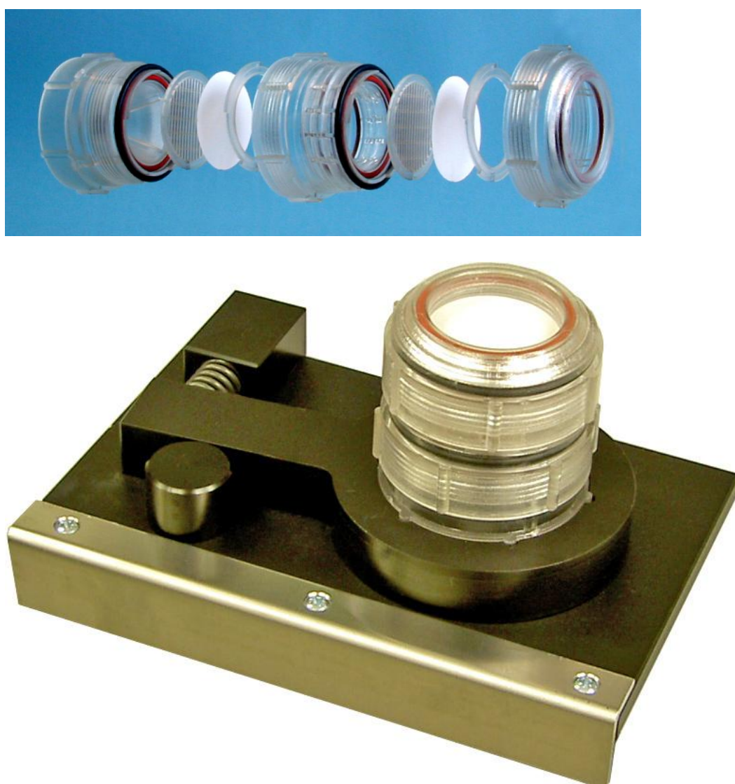
Figure 1: Filter pack with one aerosol filter and one impregnated filter for gases.
