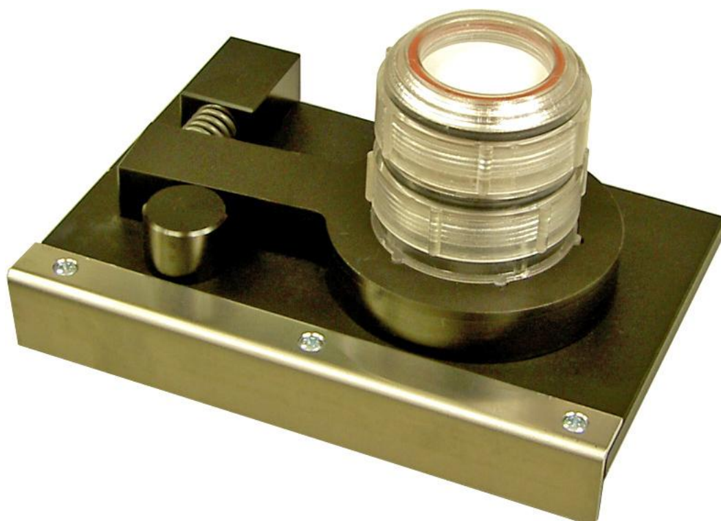
Figure 1: Filter pack with one aerosol filter and one impregnated filter for gases.
